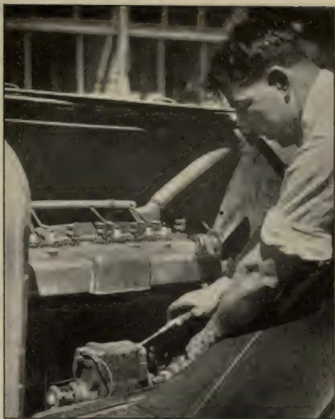
FIG. 118. The magneto in an automobile is a small dynamo.
